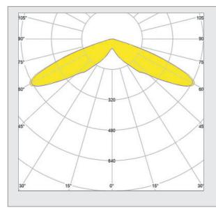
Light distribution: IESNA Typ 5-sqare measured with Philips Fortimo FastFlex LED 4x16 DHE G4
