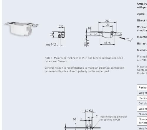
SMD-Push through terminal block with push wire contacts
