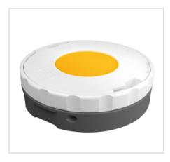
The compact module comprises a socketed and encapsulated LED lamp, together with a suitable lampholder incorporating a twist & lock fixing. The lampholder gets easily assembled with two standard screws. With the support of two preloaded leaf springs, a defined contact pressure of the light source to the heat sink ensures a reliable heat dissipation.
