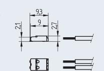
General note: It is recommended to make an electrical connection between both poles of each polarity on the solder pad.
