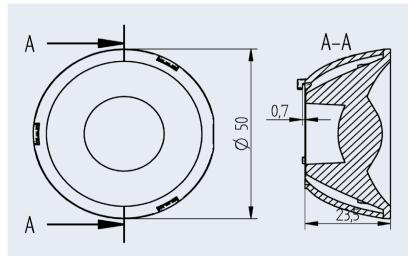
Specification Top diameter 50 mm Height 23,50 mm Material holder PC Material lens PMMA Operating temperature - 40°C ... 80°C\* Weights 30,8 g Light distribution Medium Beam angle\* (FWHM) 27° Efficiency\*\* 88,4% Recommended COB Type Citizen CLU02J
