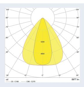
Light distribution: Oval measured with Philips Fortimo FastFlex LED 2x6 / 740 DA HE
