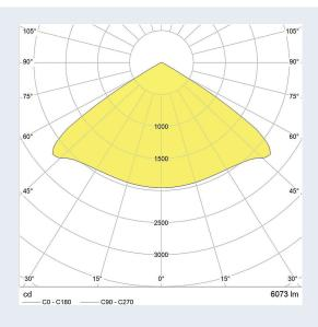
Light distribution: Extra wide measured with Philips Fortimo FastFlex LED 2x6 / 740 DA HE
