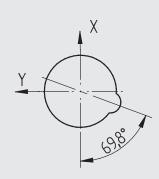
Electromechanical interface for outdoor luminaires according to Z Zhaga Book 18 to accommodate communication and sensor units
