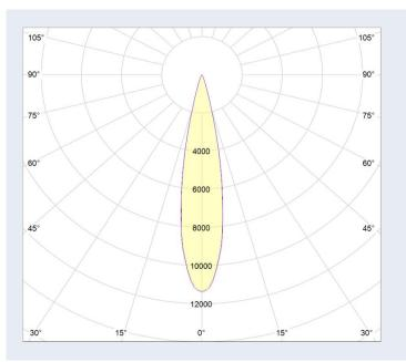
Beam angle (FWHM) measured with Luminus CHM-6 and connector 47.360.1020-0
