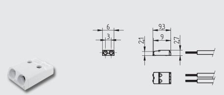
SMD-Terminal block - Nano with push wire contacts and contact opening function
