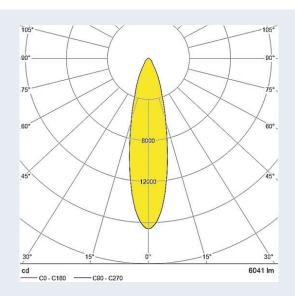
Light distribution: Narrow measured with Philips Fortimo FastFlex LED 2x6 / 740 DA HE
