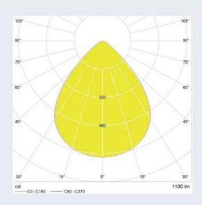
Light distribution: Wide measured with Philips Fortimo FastFlex LED 4x16 DHE G4
