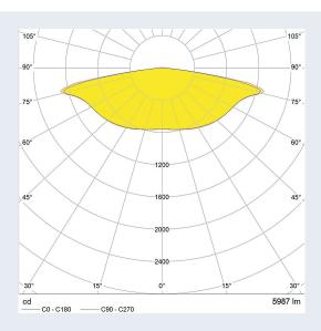
Light distribution: IESNA Type 5 measured with Philips Fortimo FastFlex LED 2x6 / 740 DA HE
