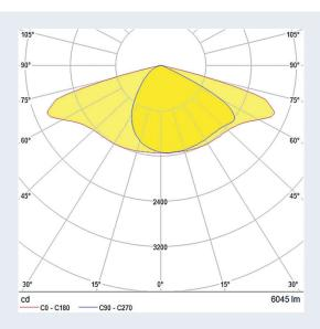
Light distribution: IESNA Type 3 M Cutoff measured with Philips Fortimo Fast Flex LED 2x6 / 740 DA HE
