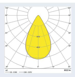
Light distribution: Medium measured with Philips Fortimo Fast Flex LED 2x6 / 740 DA HE
