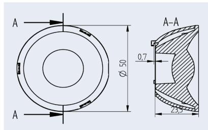
SpecificationTop diameter50 mmHeight23,50 mmMaterial holderPCMaterial lensPMMAMax. temperature80°CWeights30,8 gPkg.
