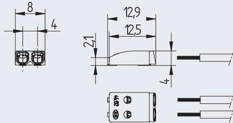
General note: It is recommended to make an electrical connection between both poles of each polarity on the solder pad.
