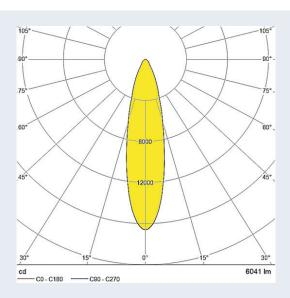
Light distribution: Narrow measured with Philips Fortimo Fast Flex LED 2x6 / 740 DA HE
