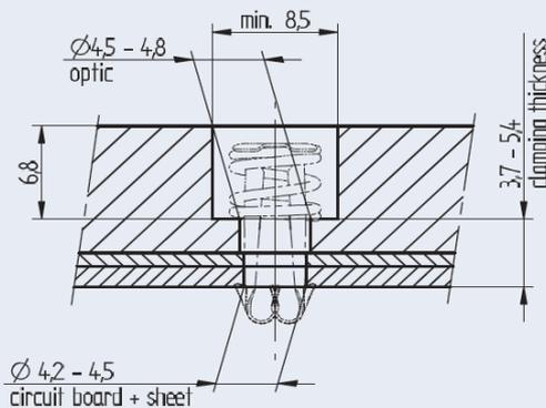
3 x 11 Optics with pre-fixed fixing element
