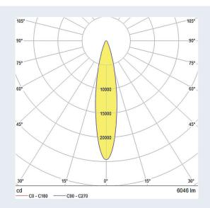
Light distribution: Ultra narrow measured with Philips Fortimo FastFlex LED 2x6 / 740 DA HE
