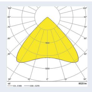
Light distribution: Wide measured with Philips Fortimo FastFlex LED 2x6 / 740 DA HE
