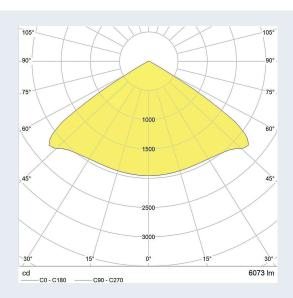
Light distribution: Extra wide measured with Philips Fortimo Fast Flex LED 2x6 DA HE
