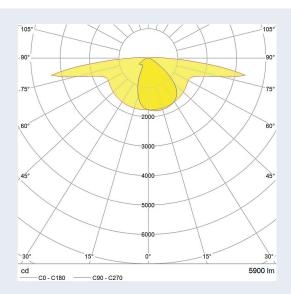
Light distribution: IESNA Type 3 Long measured with Philips Fortimo FastFlex LED 2x6 / 740 DA HE
