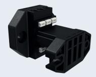
Mains voltage disconnect terminal blocks are designed to automatically disconnect the internal wiring from the main supply inside the street lighting fixture. This will help the technicians to safely do cleaning/maintenance of the luminaire.
