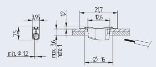
Note 1: Maximum thickness of PCB and luminaire heat sink shall not exceed 3.6 mm.
