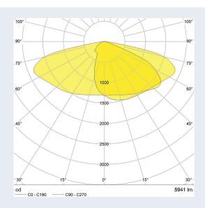
Light distribution: IESNA Type 4 Medium measured with Philips Fortimo FastFlex LED 2x6 / 740 DA HE
