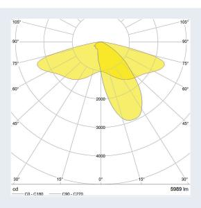
Light distribution: M-Class, IESNA Type 2 measured with Philips Fortimo FastFlex LED 2x6 / 740 DA HE
